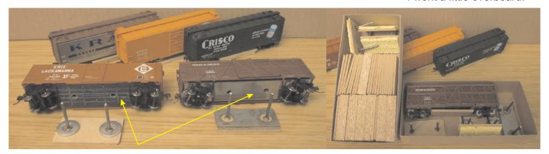
Underframe is modified to make clearance for pad.
