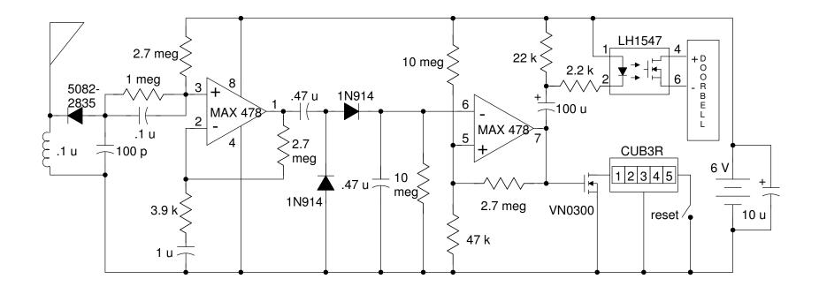
The 0.1 uH choke may be attached to antenna at any point to ground. The value is not critical.
