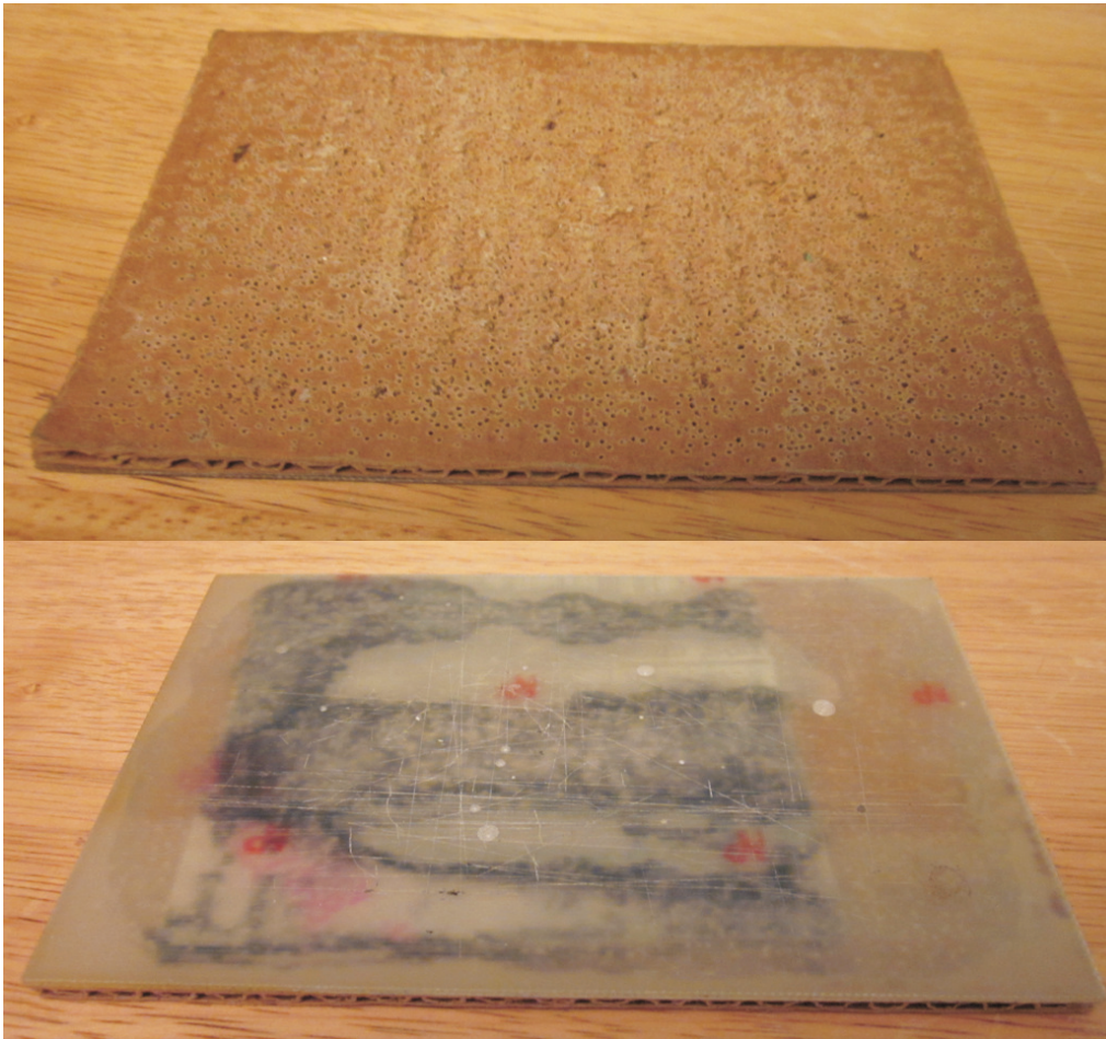
PCB with no foil. Dark areas are where the glue cause the ink on the shipping label to bleed.
