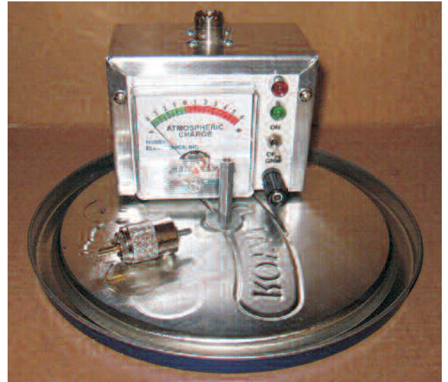
The detector and antenna parts. The connector is made by filing down a long screw to fit into the jack and soldering it. Fill the jack with epoxy up to the top. In this case a nut was added as a stop for the hex stand-off which is screwed to the cookie tin lid.
